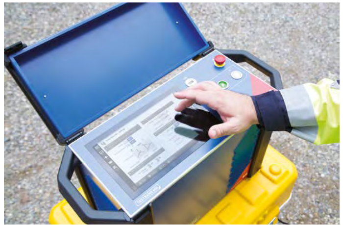
Figure 19. TESTRANO 600 – three-phase test system
